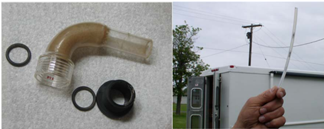
Figure 7.7 Examples of contaminated tubing and manifolds needing more frequent maintenance
