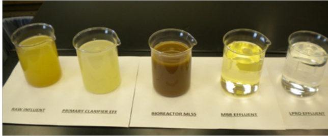
Figure 2 Water at Various Stages of the Treatment Process (Photo credit: Frito-Lay)
